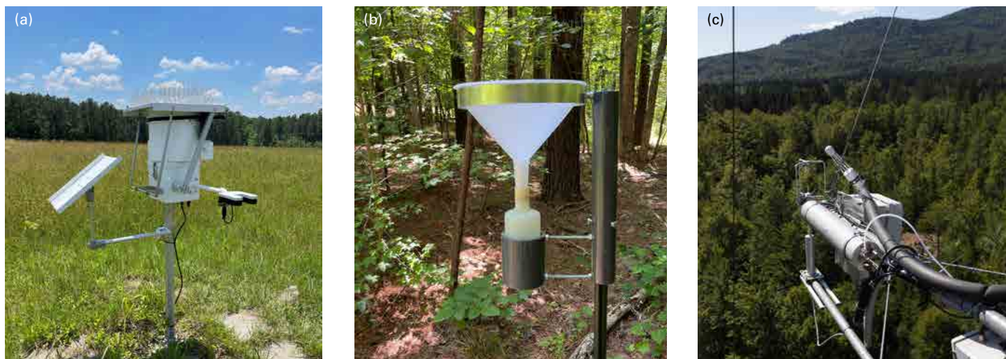
Figure 7. Examples of samplers for wet deposition ((a), Duke Forest, Chapel Hill, North Carolina, USA; photo: John Walker), wet and dry deposition (throughfall) beneath a forest canopy ((b), Duke Forest, Chapel Hill, North Carolina, USA; photo: John Walker), and dry deposition of total reactive N ((c), Bavarian Forest National Park, Germany, Wintjen et al., 2022; photo c/o Christian Brümmer). Methods for monitoring deposition range in complexity and cost, from relatively simple funnel type collectors for measuring throughfall, to the advanced systems that combine measurements of atmospheric turbulence and chemistry at higher temporal resolution that are needed to directly determine dry deposition (c).
